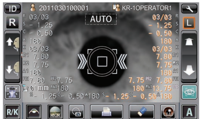
Figure 2: The KR-1 features fully automated measurement and Topcon's rotary prism technology for enhanced accuracy. All measurements are displayed on the color touchscreen for added operator convenience.
